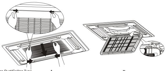
For Duct/Ceiling Type A B Push the grill switches to the arrow directions , then open the air-in grill downwards. Turn back the air filter fixing block, •then take out the air-in grill.
