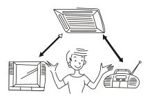
Put the TV or radio away from the heat pumpr at least 1 meter, or signal will be interfered.
